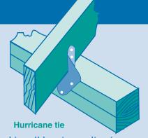
and install hurricane clips/straps to connect roof rafters/trusses to side walls (especially for gable end walls). Consider using a double layer of roofing felt, one layer of tear resistant synthetic underlayment or an adhesive backed waterproofing membrane underlayment. Ensure the roofing is installed based on the manufacturer's high wind installation instructions.
