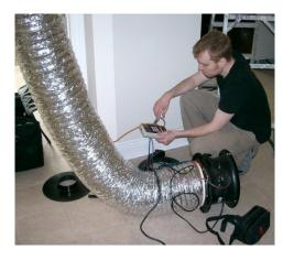
crucial air sealing techniques to achieve the 2009 IRC energy code air tightness and duct testing provisions.
