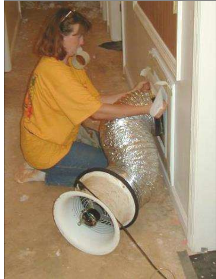
Duct Blower or Duct Leakage Tester ( Duct Blaster® )
