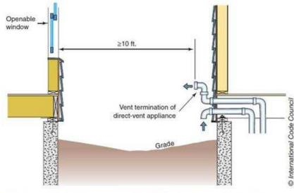
A minimum 10-foot horizontal separation is required between a vent terminal and an opening of an adjacent building.
